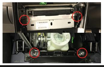
Once the main dashboard panel has been removed, proceed to undo the 2x recessed Torx screws either side of the main head unit, and the 2x screws down by the centre console.
