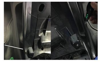
Before trying to pull out the inner trim, on the back of the inner dashboard frame are 2x screws. Remove these and then gently pry the inner frame away from the dash.
