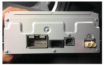
With the inner trim removed, proceed to pull the main head unit out and disconnect all of the wiring.
