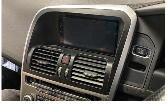
Once the stereo is secured, take the new fascia and place over the top, reconnecting the hazard switch in the process.
