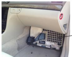
Remove panel to gain access to CAN Hub
