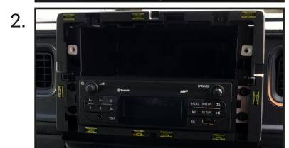
With the trim out of the way, undo the 4x screws that surround the main head unit and remove it whilst disconnecting all of the wiring.
