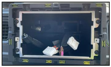
Using the 4x pre-existing screws from the main head unit, screw the frame bracket into place.
