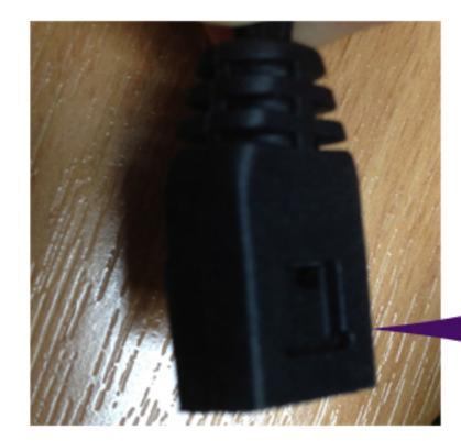
To identify the way the connector connects to the radio, the cut out indicates the bottom of the connector
