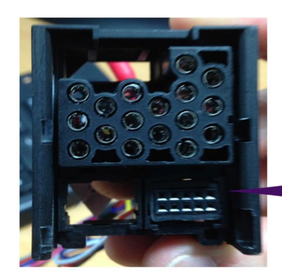
If the large connector is plugged into ther radio then the small connector will go in the left hand connector of the radio. The diagrams shows both the connector side and the wire side
