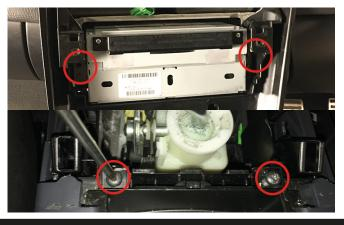
Once the main dashboard panel has been removed, proceed to undo the 2x recessed Torx screws either side of the main head unit, and the 2x screws down by the centre console.
