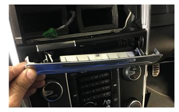
Disengage the CD slot plastic housing by bending in the clips on either side with a panel removal tool.
