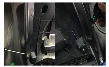
Before trying to pull out the inner trim, on the back of the inner dashboard frame are 2x screws. Remove these and then gently pry the inner frame away from the dash.
