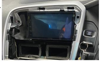
With the brackets affixed to the correct sides of the stereo and the dashboard modified, connect up the stereo and slot into place, screwing into place using the pre-existing screws.
