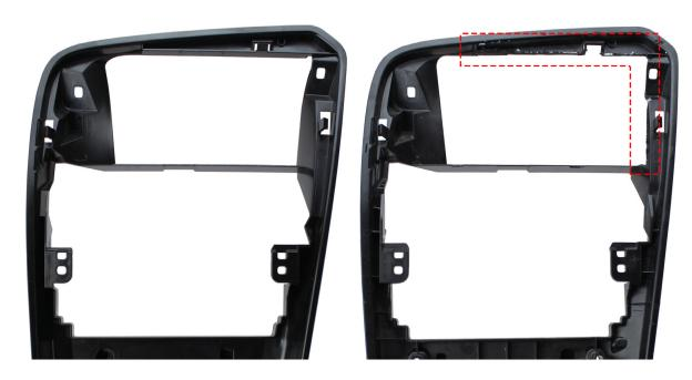
The highlighted section of dashboard frame will need to be cut in order to allow for a new double DIN unit to sit in place correctly.
