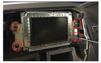
Remove the 4x screws that surround the top screen and remove completely whilst disconnecting all of the wiring.
