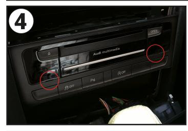
Using a pair of radio release keys (e.g. **CT22AU01**) remove the head unit. When free, disconnect all the wiring.
