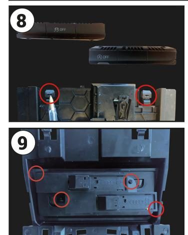
Take the OEM head unit in hand and gently remove the buttons by means of releasing the surrounding plastic.
