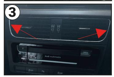
Using a pick tool, insert it in between the fan blades and release the spring clips.
