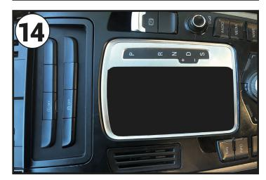
With the Button Relocation Panel fully connected and in place, begin to re-introduce the gear panel back into the dashboard.
