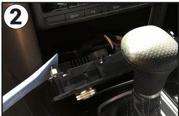
Using the Bojo tool again, pry away and unclip the bottom HVAC panel.
