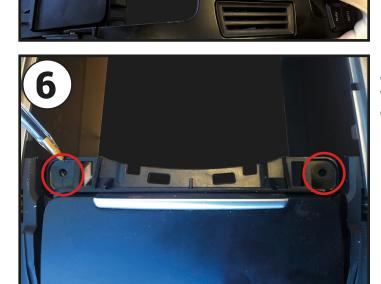
Remove 2x 8mm screws located toward the bottom of the ashtray panel (*see image reference*). When free, carefully lift and pull the ashtray pocket up out of the dashboard.
