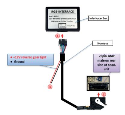
**Note**: If the 26pin AMP-socket of the head-unit is already occupied, the vehicle may have a factory TV-tuner. It must be removed to complete installation. To do so, disconnect the female 26pin AMP-connector of the factory harness and disconnect all wires from the factory TV-tuner.
