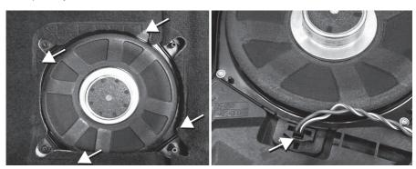
Remove the screws from the subwoofer and unplug the connector from the subwoofer. Press the tab on the connector to unplug. Sometimes it's easier to lift up the subwoofer, before unplugging the connector.
