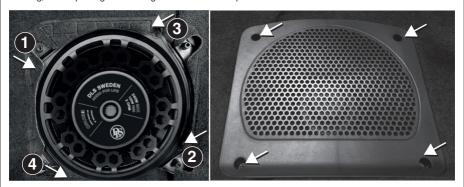
Plug the OEM connector in the DLS subwoofer. Mount the subwoofer in the housing. There is a dowel pin by the connector for lining up the subwoofer. Make sure the connector is still fixed.
