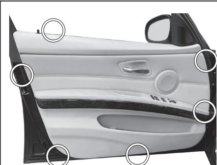
Loosen the door panel by inserting the pry tool between the panel and the door. Pry the door panel gently, but firm, outward to release the clips.
