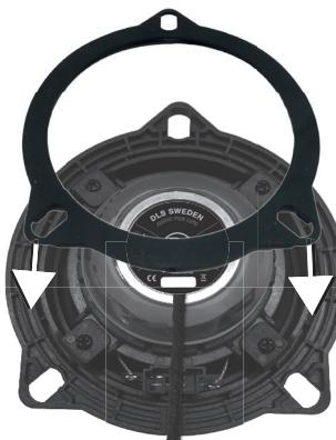
Mount the foam gasket (115mm x 4mm) on the top of the basket. Peel off the protective cover of the adhesive tape. Press firmly all around the foam gasket to make it stick properly.
