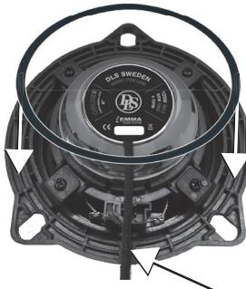
Mount the foam gasket (115mm x 13mm) on the top of the basket. Peel off the protective cover of the adhesive tape. Press firmly all around the foam gasket to make it stick properly.
