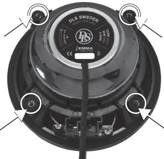
Place the plastic adapter over the speaker and fix the frame with four included screws.
