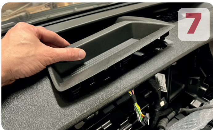
Take out the top storage. ! Note : if your Transit is equipped with a tablet or smartphone holder, you need to replace it with this holder. Ford ref. : 2364170
