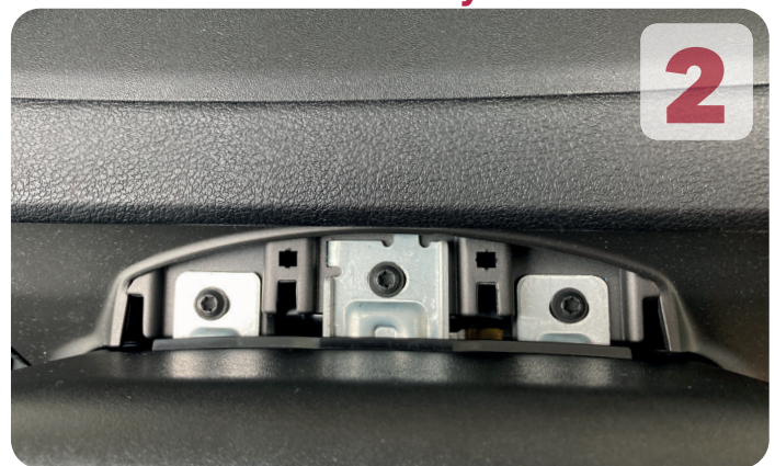
Remove the cover right behind the top of the screen and remove the three screws.
