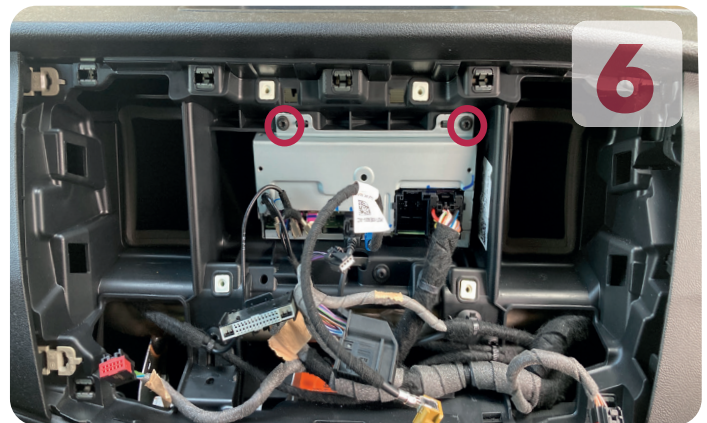
Remove the connectors and two screws to take out the original control unit.
